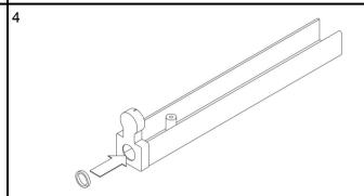
• Insert supplied Ø20mm grommet into hole.
