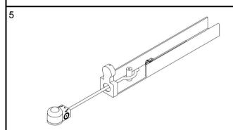
Feed cable through end-cap knockout or between gear tray and housing of luminaire.
